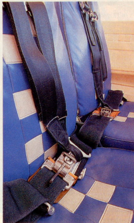
The wing struts are larger on the Aerobat, and the four-point harnesses are appreciated during aerobatic maneuvers. Jettisonable doors and two slip indicators, one on either side of the panel, are also unique features of the aircraft.
