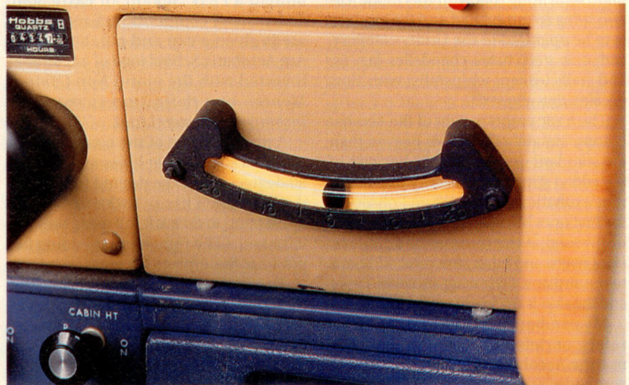
The wing struts are larger on the Aerobat, and the four-point harnesses are appreciated during aerobatic maneuvers. Jettisonable doors and two slip indicators, one on either side of the panel, are also unique features of the aircraft.
